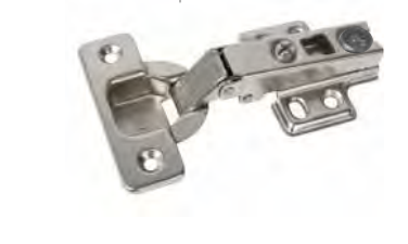
ITEM 984 | 110° FULL OVERLAY CLIP ON HINGE WITH BASE PLATE RIH520
