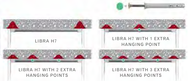
DRILLING PLAN WITH BACK PANEL WOOD THICKNESS 4MM AND H. 80,5MM ALUMINIUM BAR
